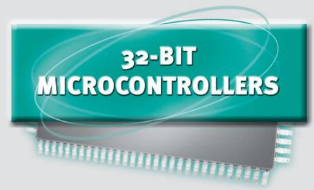
The TC10GP is the industry's first single-core 32-bit microcontroller-DSP based around the Infineon TriCore-1 architecture. The TC10GP implements the computational capabilities of DSPs alongside the most optimized price/performance implementation of a RISC load/store architecture. It is well-suited for a wide variety of real-time oriented embedded control systems.
