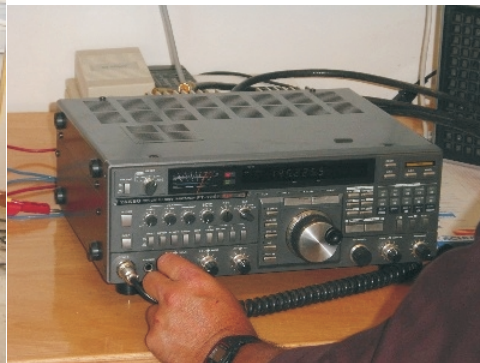
2m/70cm Transceiver, YAESU FT 736
