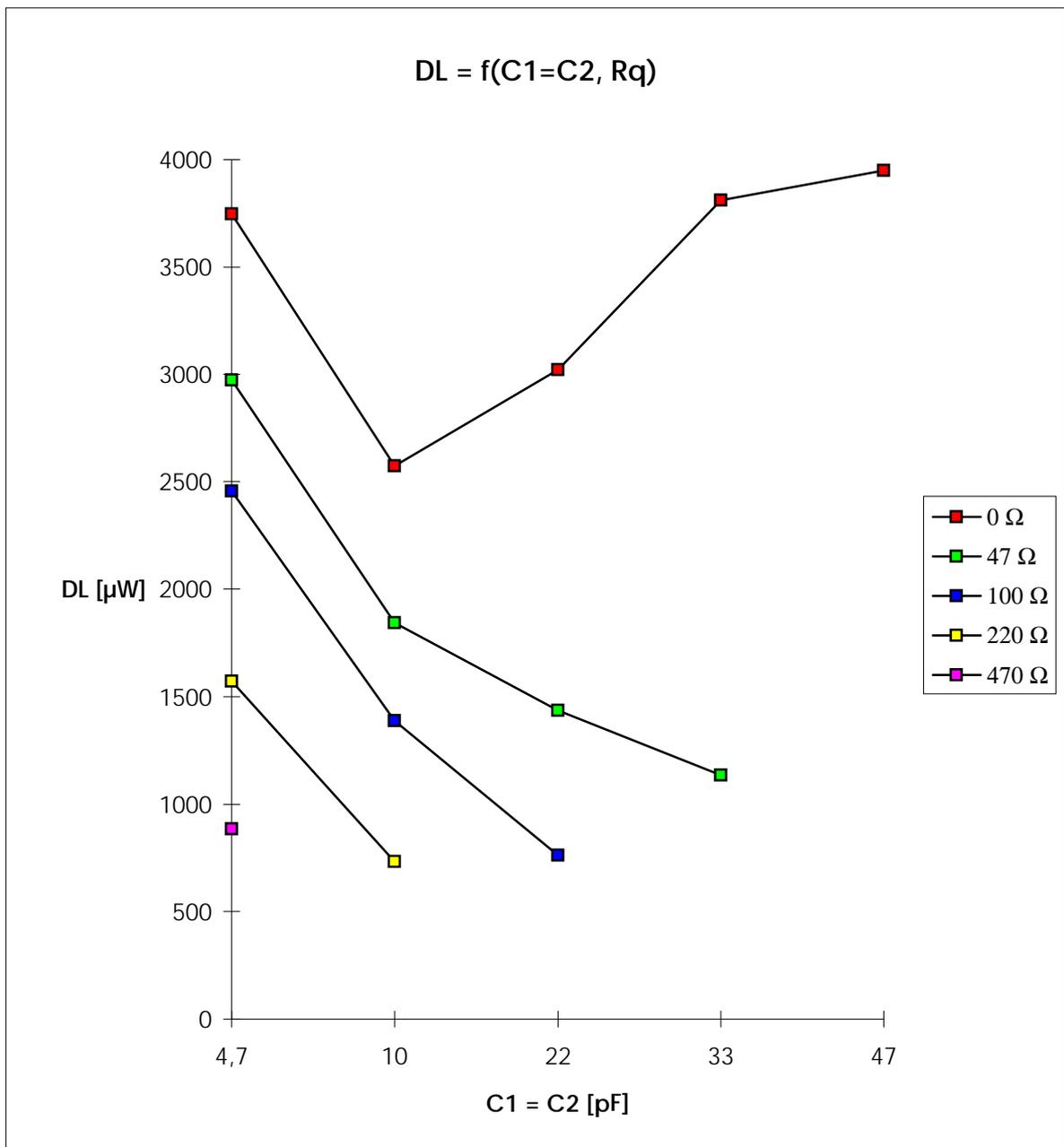
Drive level dependent of Rq and the load capacitors C1/C2
