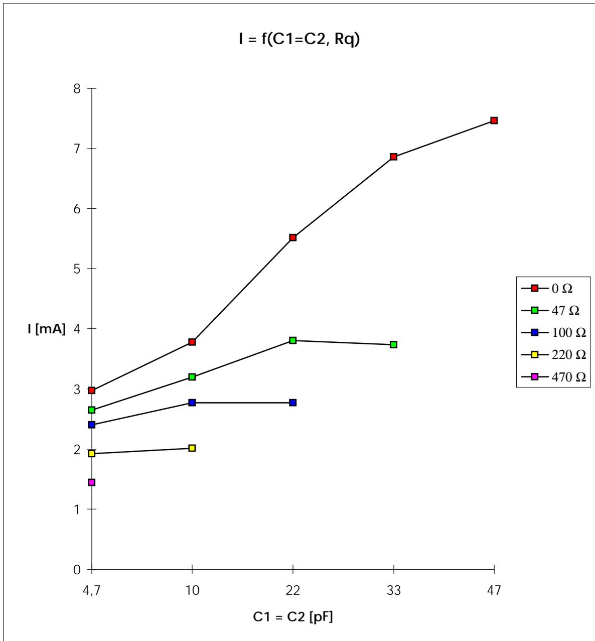
Drive current dependent of Rq and the load capacitors C1/C2
