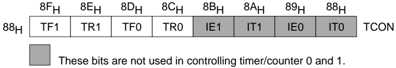
Figure 7-19 Special Function Register TCON (Address 88H)
